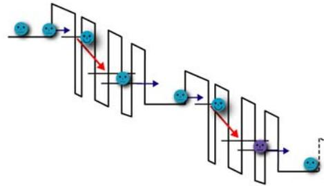
When applying an electric field, the overall downward trend of energy produces coherent photons of like kind and wavelength.<sup>3</sup>
