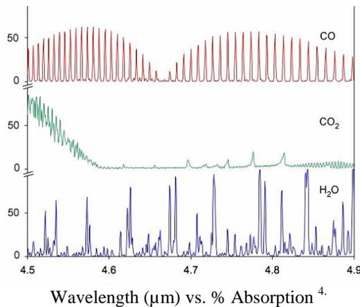
Fundamental absorption wavelengths for the combustion gases of CO, CO<sub>2</sub> and H<sub>2</sub>O are in the mid-Infrared, which makes the Quantum Cascade Laser the natural fit for the analysis.
