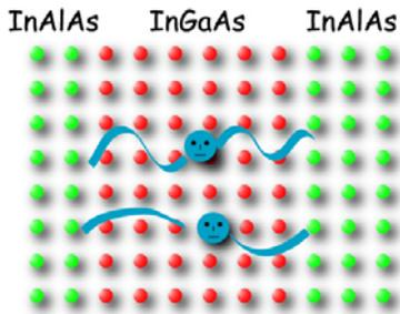
There may be over 100 layers of semiconductor material which may be as small as 0.3nm (layers of atoms).<sup>3</sup>
