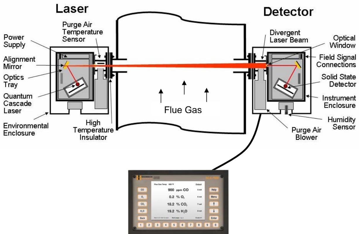
The Transmitter provides local readouts of the gas concentrations, setup parameters and other process information. Complete analyzer diagnostics, averages and fault histories also are available.
